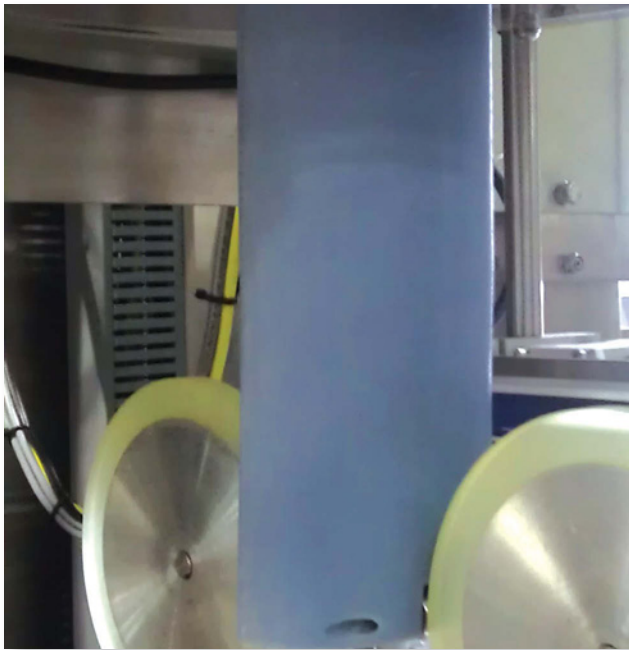
Close-up of shrink-sleeve tooling built on Objet Eden 260V additive manufacturing system, for Axon Styrotech shrink-sleeve packaging equipment. Image courtesy of Axon Styrotech.
