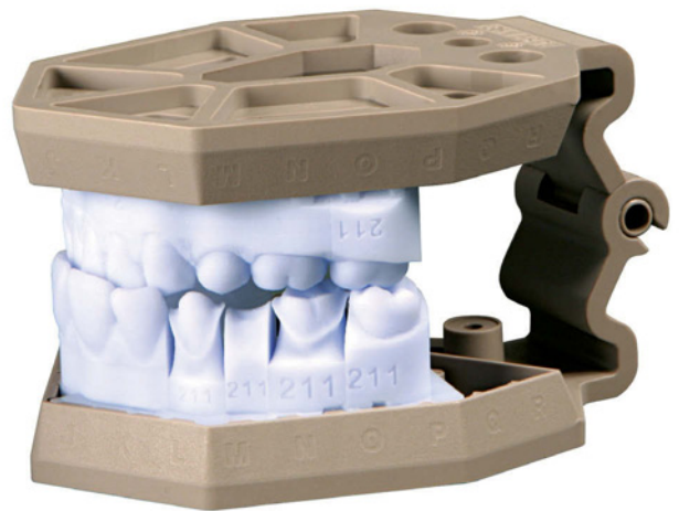
Dental models in a custom proprietary SLA resin built by In'Tech Industries on a fleet of 3D Systems' IPro 8000 and 9000 SLA machines. Image courtesy of In'Tech Industries.
