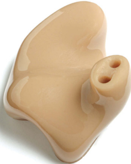
Hearing-aid ear shell built by In'Tech Industries on 3D Systems' Viper Si SLA system, with thousands built daily. Biocompatible material is Dreve Fototec; gloss finish is net-proprietary finished (no post-polishing or lacquering). Image courtesy of In'Tech Industries.
